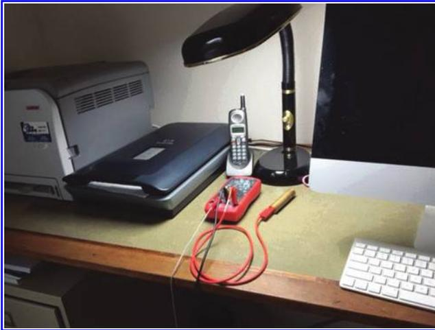
**FIG. 1.** Experiment setup with from left to right: printer, scanner, cordless phone, lamp, computer monitor, and keyboard. The multimeter is the red instrument in front of the phone and lamp.
